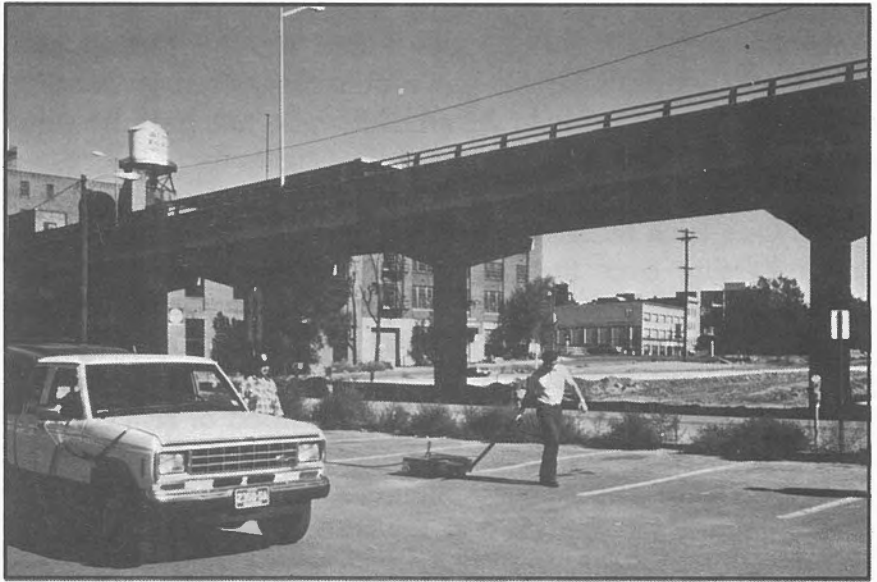
Figure 7 - Ground-penetrating radar test in progress. The towed sled contains transmitting and receiving antennae, which relay an image of buried soil strata and cultural features to a printer.
