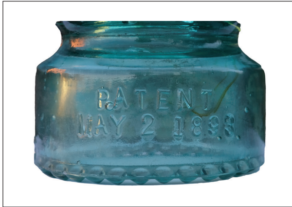
Figure 12. The patent date for drip points (May 2, 1898) embossed on the skirt of an insulator. (Photo by Joshua Birndorf.)
