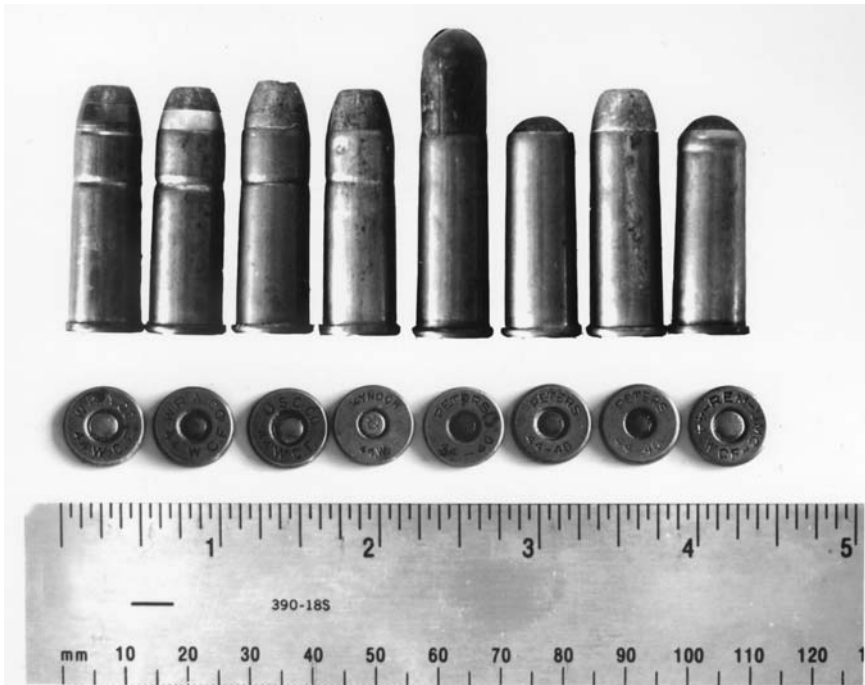
FIGURE 2. Example of variety of cartridges in the same caliber. These are all .44-40 caliber. Note differences in bullets, cases, and headstamps. Two cartridges on left are the same, except the bullets are jacketed in different metals. Cases at right and third from right are loaded with round balls. Case fourth from right has shot enclosed in a paper “bullet.”
