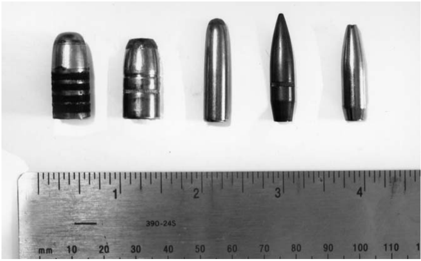
FIGURE 8. Bullet types, left to right: unjacketed lead bullet; flat nose; soft point; spitzer boat tail; hollow point.
