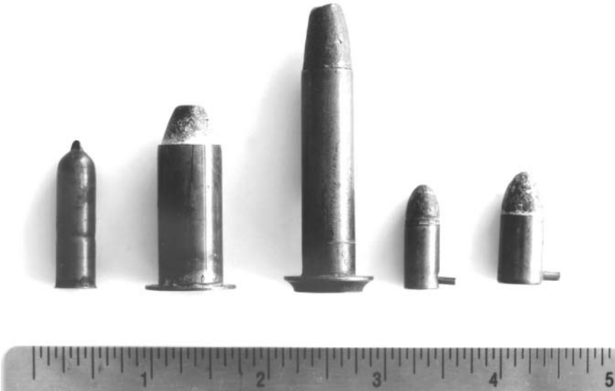
FIGURE 7. Oddities, left to right: .32 teatfire patent 1864; .50 Maynard 1865; .44-60 Maynard Model 1873 (centerfire); 7mm pinfire; .32 pinfire. Scale in inches.
